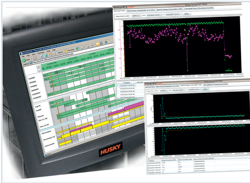
Fig. 4. With the program ShotScope NX, process data like current energy consumption are recorded over the production cycle © Schöttli/Husky
